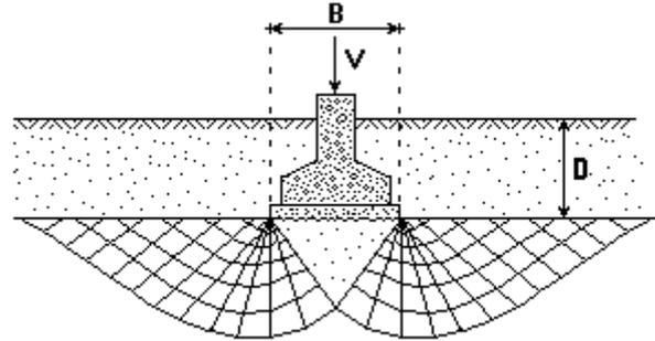
$$N_q = e^{\pi \cdot \text{tg} \phi} \cdot \text{tg}^2 \left( \frac{\pi}{4} + \frac{\phi}{2} \right) \quad N_c = \frac{(N_q - 1)}{\text{tg} \phi} \quad N_\gamma = 2 \cdot (N_q + 1) \cdot \text{tg} \phi$$
